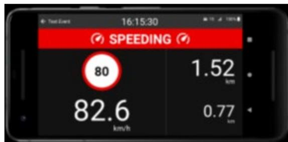
When the device detects an overspeed this device will warn the user with an audio tone and a red bar as seen in this
