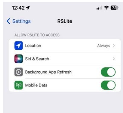
Another check – Select Location (on the RSLite settings page), make sure location services is set to always, and ensure that Precise Location is enabled.
